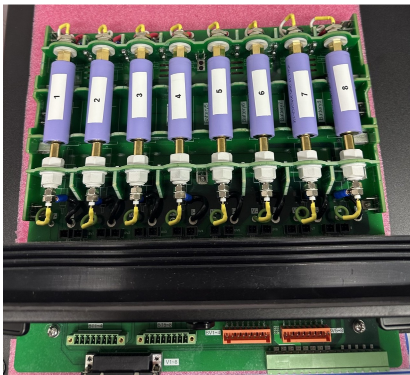
Figure 2. The eight XCell N18650CP-35E cells in the PDBT tray. Each cell has separate current-carrying and voltage-sense connections.
