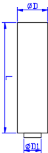
Figure 38: Battery Cell Size Specification
