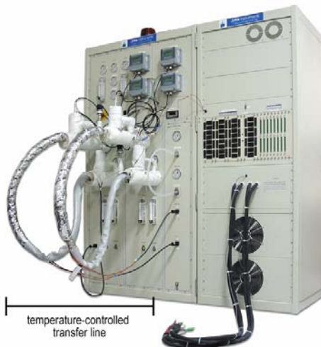
PEMFCTS-1000A/100A-0/50V-10kW-200slpm anode humidifier-600slpm cathode humidifier
