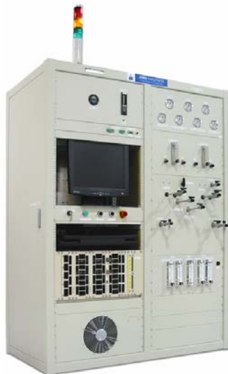
PEMFCTS-500A/5A-0/6V-1kW-20slpm anode humidifier-50slpm cathode humidifier
