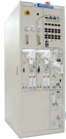
PEM/DMFCTS-1ch e-load at 50V/100A/1kW-1.3lpm methanol line-20slpm anode humidifier-50slpm cathode humidifier
