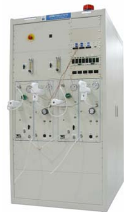
DMFCTS-2ch e-load at 2V/20A/20W-60ccpm methanol line- 2 sets of 2slpm cathode humidifier
