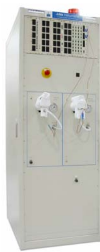
PEMFCTS-1ch e-load at 30V/100A/3kW-50slpm anode humidifier-200slpm cathode humidifier
