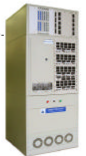
8-channel BT2000-PWM-MOSFET-((-1)V-100V)-25A/1A/0.1A, 2500W, 8 pressures, 16 thermocouples, 40 aux voltage inputs
