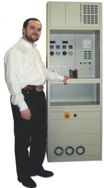
Pierre-Jean, Arbin sales engineer, stands next to a linear, high power, one channel fuel cell testing system. Voltage range from 0-30V, 100A current, and maximum power of 500W.
